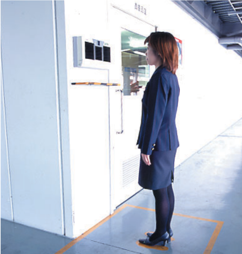
The iris camera automatically captures the pupils of the eyes when a person stands facing it. Identification is completed without touching anything.
